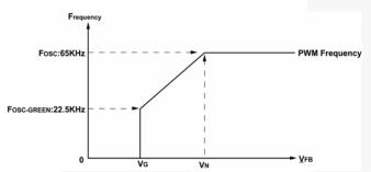
Figure 7. PWM Frequency vs. FB Voltage
