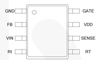
Figure 1. Pin Configuration
