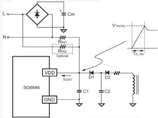
Figure 6. Circuit Providing Power
