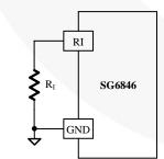
Figure 5. Setting PWM Frequency
