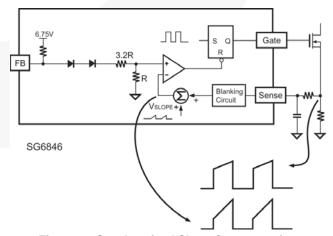
Figure 9. Synchronized Slope Compensation
